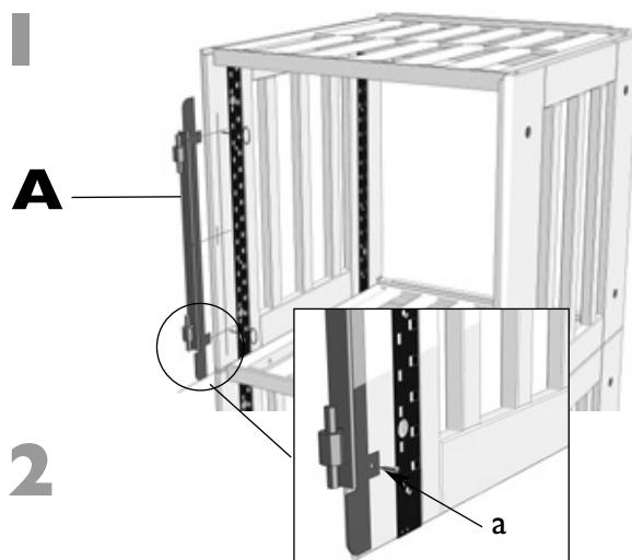
1 : Position the hinge (A) so that the lower part is lined up with the upper corner of the shelf.
