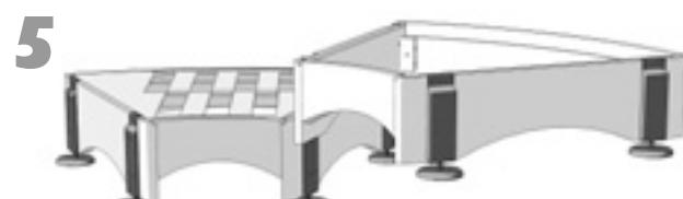
**5**: Line up the holes and insert the 2 screws (**a**) in the remaining free holes in each foot support.
