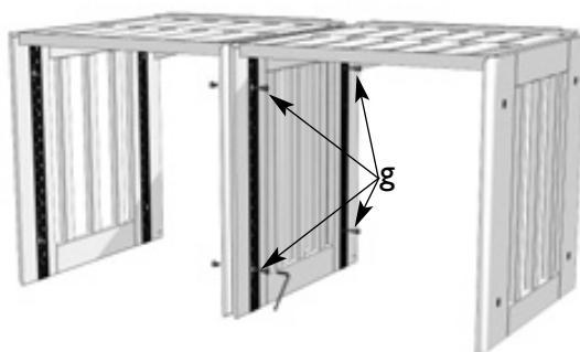
**3:** When the 2 modules abut, you will need to link them using 4 linking screws (g). Push the linking screws into the holes provided in the shelf support strips on the 2 contacting panels. Tighten until the 2 panels are flush and in line.
