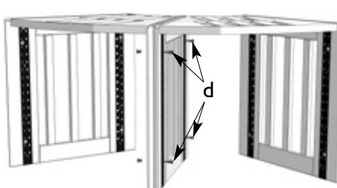
**3** : When the 2 modules are back to back, you will need to link them using 4 linking screws (d). Push the linking screws into the holes provided in the shelf support strips on the 2 contacting panels. Tighten until the 2 panels are in contact and correctly aligned.
