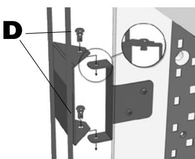
4 : Position the bottle holder on the securing tab, insert the 2 rivets (**D**) and fit by exerting light pressure on each of them.
