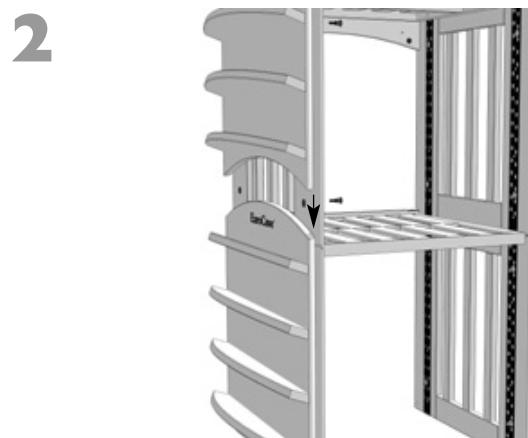
**2**: Place the bottle holder on the one below, and secure it using the 4 linking screws and tighten from inside the basic module.
