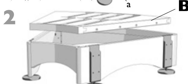
**2**: Place the module on the floor and check the height of pedestal using a spirit level.
