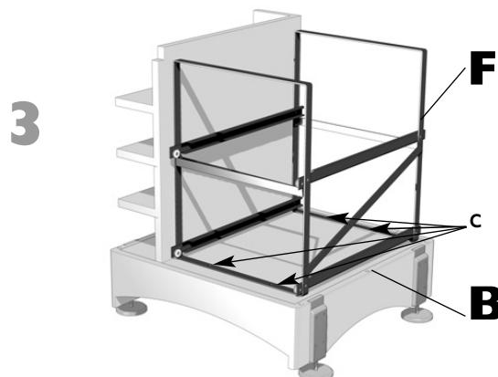
4 : Position the upper cross piece (C) under the rack of the basic module and position it on the edge of the rack, securing it with 3 screws (a).
