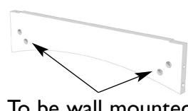
**4:** The basic modules above the first should be secured to the wall from the 2<sup>nd</sup> level using 2 securing screws (not supplied) suitable for the wall type..
