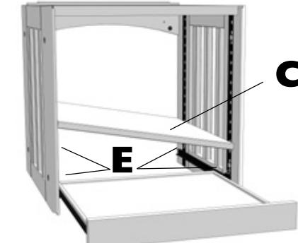
**3** : Position the 4 shelf supports (**E**) in the shelf support strips and set up the shelf (**C**).
