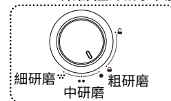
(註 1) 研磨粗細調節旋鈕
